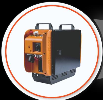
**CONTROLLER INTEGRATED INTO THE ROBOT BASE**
