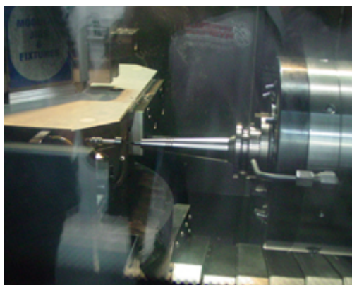
Renshaw tool setting probe in action
